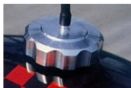
Detailverliebt: CNC-gefräster Tankdeckel in Originalform
